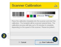
To perform scanner calibration, click the Start Calibration button (1). Status messages and a progress bar will keep you informed about the process (2).
