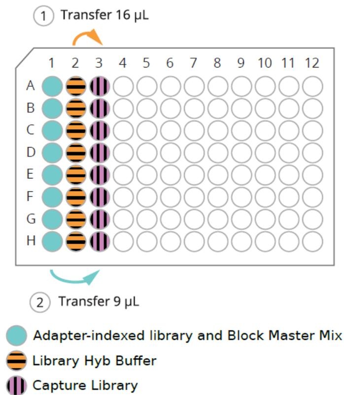
Figure 3. Overview of final plate setup
