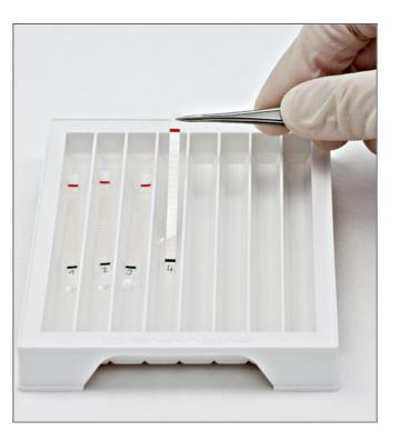
Incubate for **30 min** at **45°C** on the shaking platform of the waterbath or thermoshaker.
