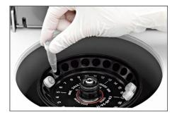
Centrifuge for **5 min** at **12,000 rpm** in a microcentrifuge. Cool on ice.
