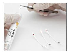
Label Teststrips outside of the marker lines with a pencil. (No ballpoint pens, ink markers, etc.)
