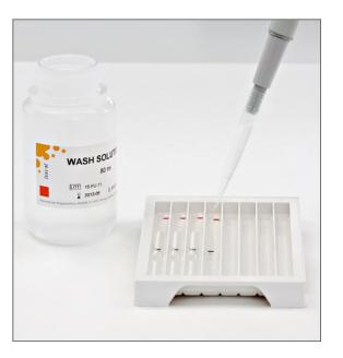
Add **1 ml Color Developer**. Incubate for **15 min** at **room temperature** <u>in the dark on a rocker or orbital shaker</u>.
